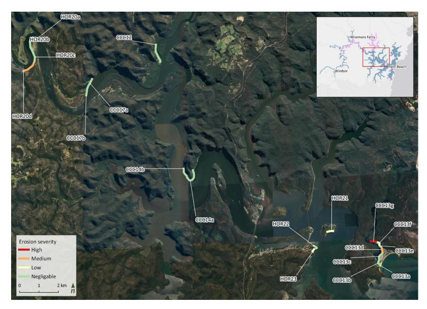
Figure 18. Erosion severity at the full bank erosion assessment sites between Singletons Mill to Patonga
