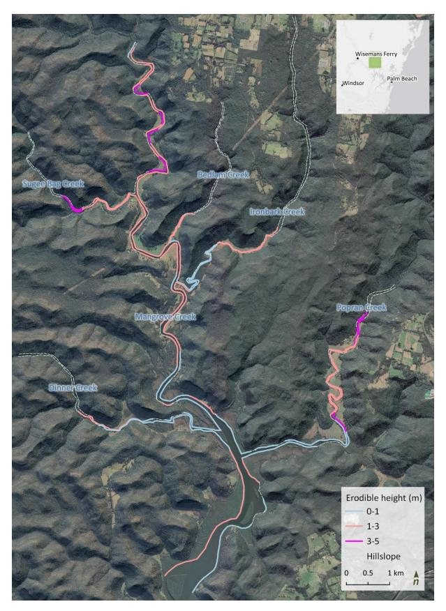
Figure 13. Erodible height (bank height) across the streambanks within the CCC11 site.
