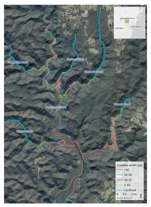
Figure 12. Erodible width (confinement) across the streambanks within the CCC11 site.
