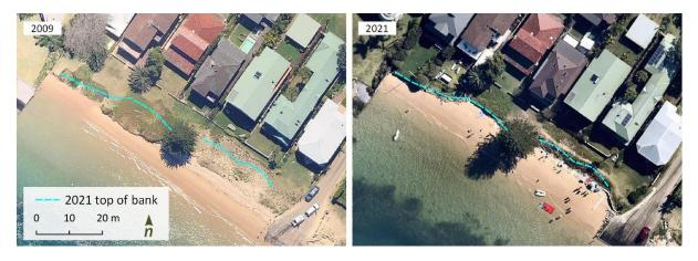
**Figure 5.** Multi-temporal aerial imagery analysis at Sand Point Beach, Pittwater, showing up to 10 m of bank retreat between 2009 and 2021.
