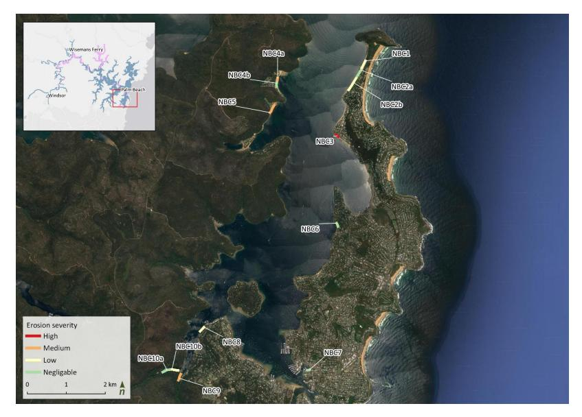
Figure 19. Erosion severity at the full bank erosion assessment sites within Pittwater Estuary
