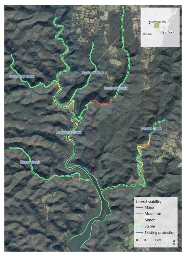
Figure 15. Lateral stability across the streambanks within the CCC11 site.
