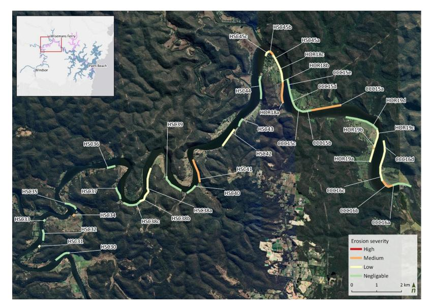
Figure 17. Erosion severity at the full bank erosion assessment sites between Portland and Laughtondale
