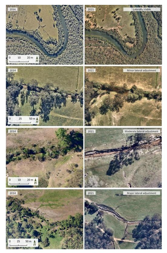
**Figure 10.** Examples of multi-temporal analysis for each of the lateral stability categories (Top two comparisons image from Popran Creek, Bottom two comparisons from Ironbark Creek).
