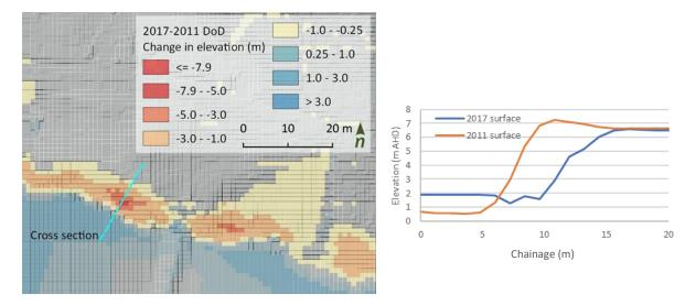
Figure 7. Example of DoD analysis between 2017 and 2011 on the Hawkesbury River at Holmes Drive Reserve. Cross section comparison of bank morphology shown on right.
